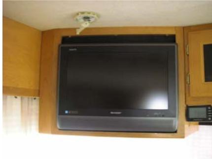
1. Using a hex wrench, loosen the set screw on the UHF Antenna and remove the crank, spring and plastic insert. Set aside for later reinstallation.
