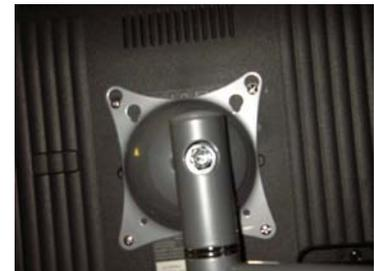
13. With the mount attached, check to see if the TV easily swings out of the way and adjust the four Adjustment Nuts accordingly.
